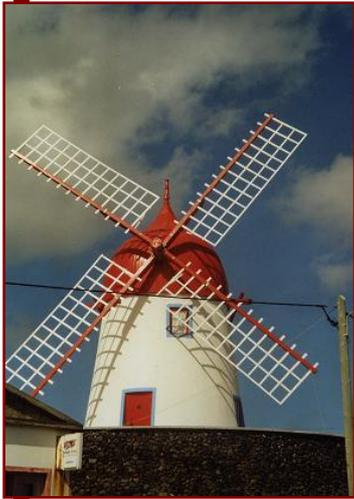
◀ This “Dutch “ style windmill sometimes has a conical versus domed rotating roof and has 4 cloth-covered sails. The wooden semi-ovoid tower sits on a stone base. The It is most common on the islands of San Miguel, Santa Maria and Graciosa.
