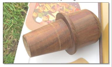
It is the bottom bearing for a turbine, made of a very hard wood, Lignum Vitae, from the Caribbean. The wood has natural oils that self-lubricate as it wears away. The turbine runner has a cup on the bottom that rests on the rounded top of the bearing. Below is a picture of a bearing as it would be positioned in the bottom frame of a turbine.
